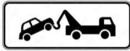
Figure 5. Additional board: Towing sign placed below a prohibition sign.
